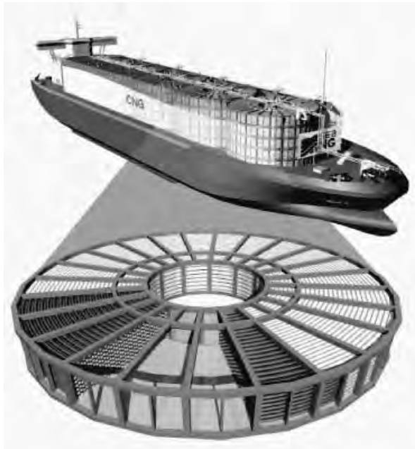
Figure 5–9 Schematic of a CNG vessel (Courtesy Sea NG Corp., 2008)
