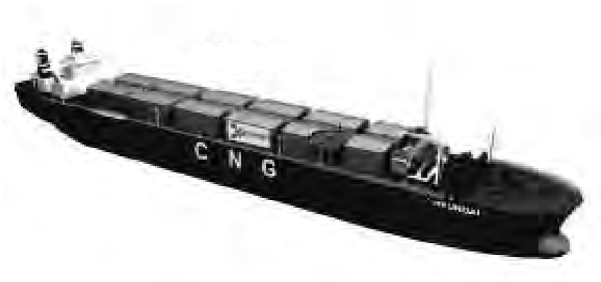
Figure 5–10 Schematic of a CNG vessel (Courtesy Enersea Transport LLC, 2008)
